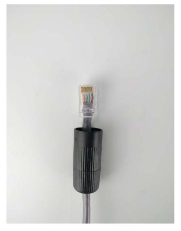
4. Plug into the Network socket of Reolink PoE IP camera and close the waterproof cover.
